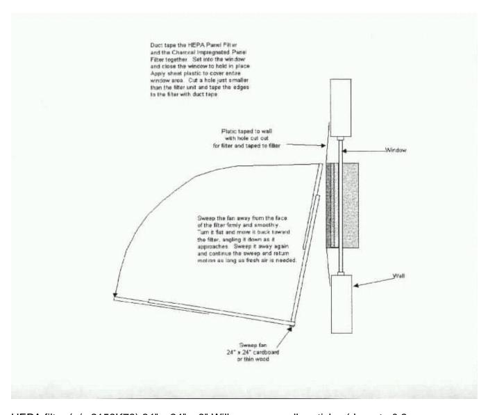
HEPA filter (p/n 2153K73) 24" x 24" x 6" Will remove small particles (down to 0.3 micron) which includes most biological contaminates
