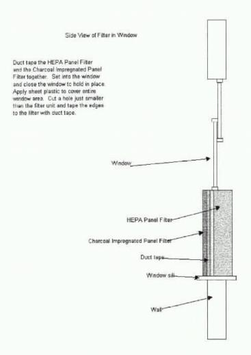
HEPA filter (p/n 2153K73) 24" x 24" x 6" Will remove small particles (down to 0.3 micron) which includes most biological contaminates
