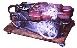
with fuse, a DC to AC power converter, a low voltage control switch, a scrap of 3/4" plywood, a few scraps of 2 x 4 lumber, 4 wheels, and two battery cables. We also used a custom designed bracket manufactured from a local fab shop to make it all come together in a snap.
