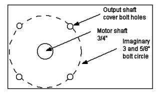
bolt holes at the base for mounting the motor to a flat surface. And the 3rd thing is that they all have four tapped holes on the output shaft cover plate. These output cover plate mounting holes are a key feature of horizontal shaft motors. Be sure the motor you purchase have them if you plan to use a bracket like the one we designed!
