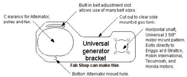
You can designed and manufactured a simple, one piece universal mounting bracket specifically for this task! This bracket bolts to the motor (using a universal bolt pattern), and allows the alternator to bolt directly to the bracket. The bracket also has an integral belt adjustment slot, which allows the alternator position to be adjusted, which serves to tension the belt.
