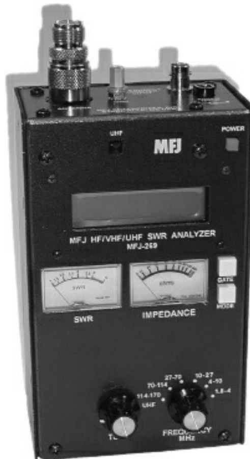
Figure 4.18 — The popular MFJ series of antenna analyzers are used to adjust and troubleshoot antenna systems. The instrument contains a low-power signal source with an adjustable frequency and an SWR meter. The LCD display shows the operating frequency and information about the antenna impedance. The meters show SWR and feed point impedance.
