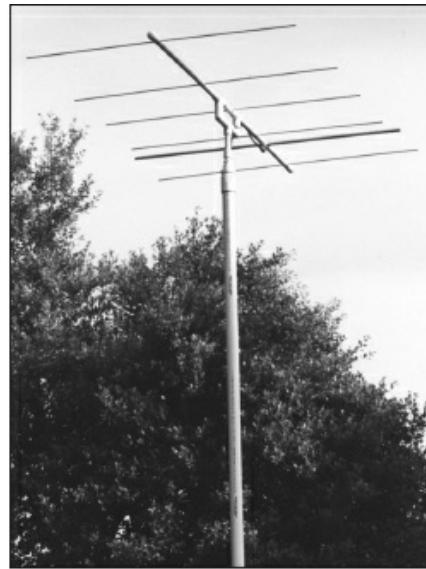
Figure 4.4 — The ground-plane antenna shown at the left radiates a signal from the vertical wire attached to the base. The vehicle's metal surface acts as an electrical mirror, creating the effect of another wire opposite to the one above the surface. On the right, the Yagi beam antenna uses parasitic elements to direct the signal in one direction and reject signals in the opposite direction.
