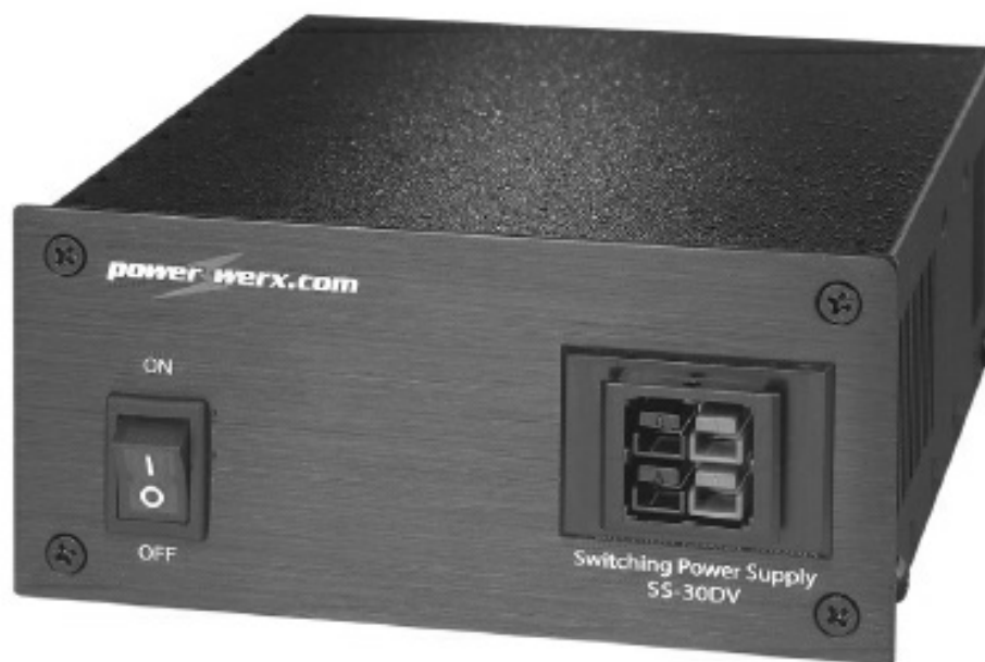
Figure 5.12 — The traditional or “linear” power supply (top) is a reliable, if heavy and bulky, performer. The modern “switching” supply shown below uses sophisticated electronics that do not need a large iron transformer, delivering equivalent power at a fraction of the weight.
