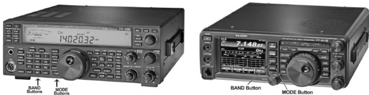
Figure 5.5 — The frequency and mode controls are shown for a pair of HF radios, the Kenwood TS-590SG (left) and Yaesu FT-991A (right). On the TS-590SG, bands are selected by pressing the appropriate button on the front panel (1.8, 3.5 and so on). On the FT-991A, pressing the BAND button brings up choices on the touchscreen display. Frequency within a band can be adjusted with the large tuning knob. If a computer is connected to the radio, frequency may be changed by the computer software. Pressing the MODE key button on the FT-991A brings up available mode choices on the touchscreen display. On the TS-590SG, there are separate mode buttons for USB/LSB, CW/FSK, FM/AM, and DATA.
