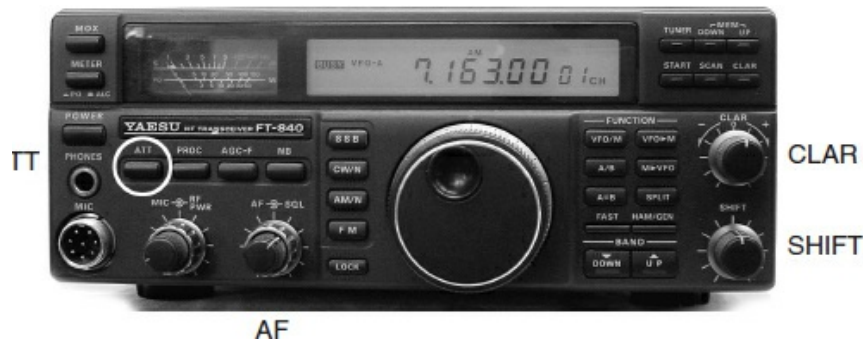
Figure 5.7 — The front panel of this Yaesu FT-840 transceiver has some of the receiver controls you'll use every day. AF GAIN (labeled AF) is the volume control. CLAR (RIT) and SHIFT vary the receiver frequency without changing your transmit frequency. ATT adds attenuation to reduce the strength of very strong received signals.
