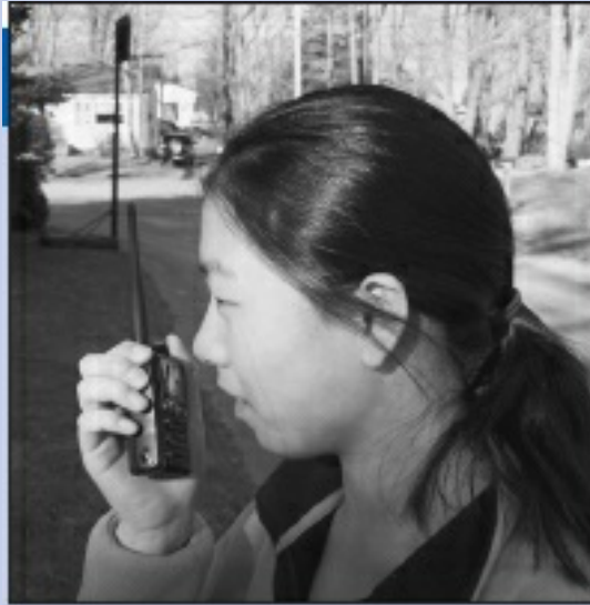
Figure 4.11 — To get the best range from a handheld radio, hold it so that the antenna is vertical. This aligns your antenna with those of a repeater or another handheld user. Also, turn the microphone slightly away from your face when talking so that your breath does not blow directly into it.
