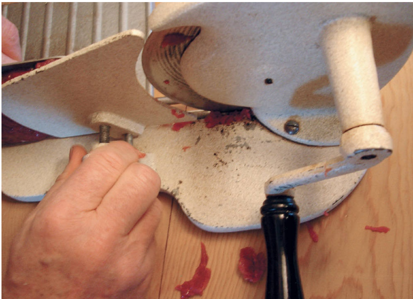
This hand slicer model has an adjustment knob on the side that allows you to increase or decrease the thickness of the meat slices.
